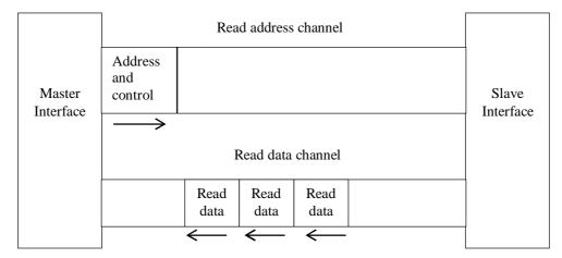
Fig. 3 Channel Architecture of Reads
