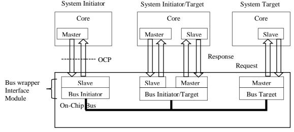
Fig.9 System with wrapped bus and OCP Instances
