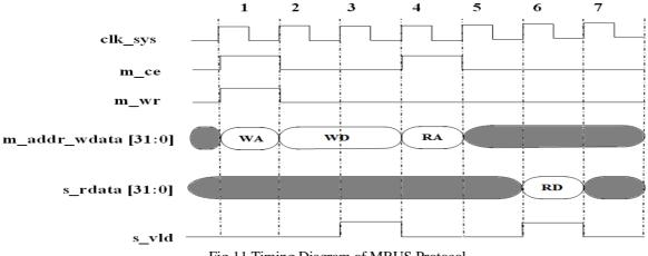
Fig.11 Timing Diagram of MBUS Protocol
