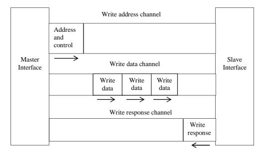
Fig. 4 Channel Architecture for Writes
