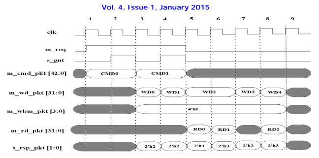
Fig.12 Timing Diagram of SBUS Protocol
