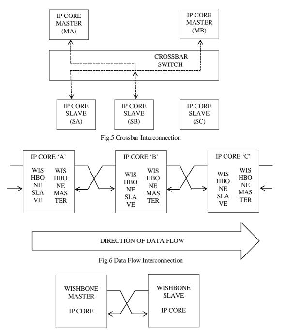
Fig.7 Point-to-Point Interconnection
