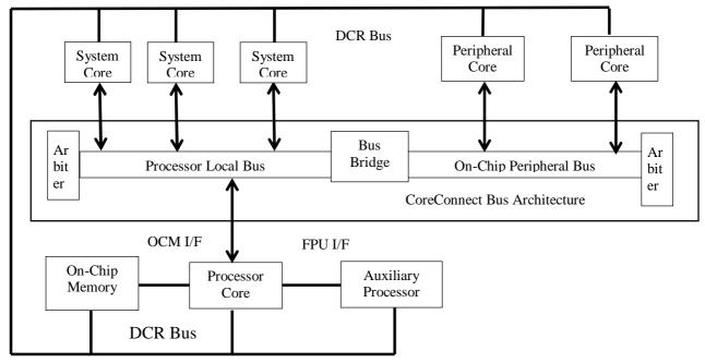
Fig.10 CoreConnect Bus Architecture
